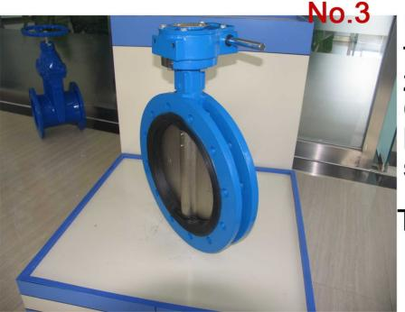
No.3 is U type butterfly valve with vulcanized seat, not replaced. OD of rubber seat is larger than NO.2 in same size.
