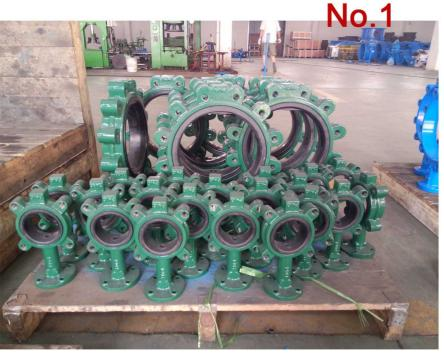
No.1 is our lug butterfly valve, seat is replacement seat with vulcanized back.
