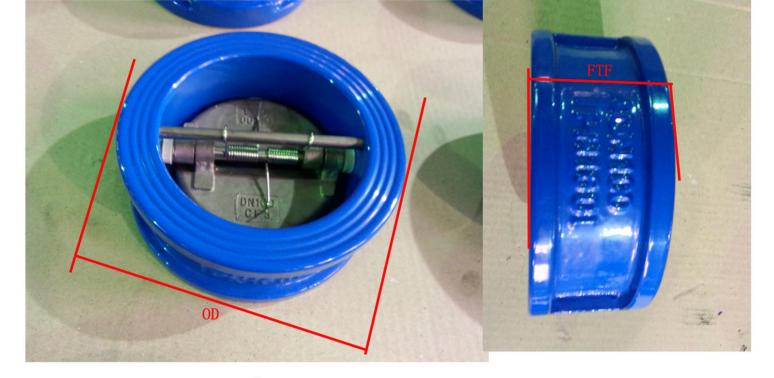
In the offer list, FTF of 3" is 64mm, OD is 142mm, it is fit to EN1092 Flanges, not fit to ANSI150.
